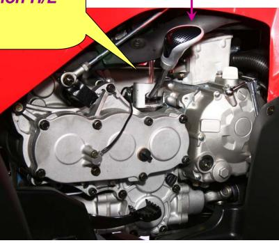
transmission gear is to get high torque application. Our design can gain about 50% extra torque in order to carry heavy load and trailer. This also increase the life time of CVT transmission system and increase engine durability.
