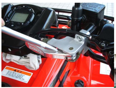
The new position of parking brake lever is the update design to prevent the driving without release parking brake
